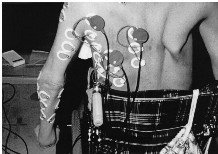
Fig. 1 Electromyography during push-up movement Each action potential was measured and recorded using silver disc electrodes, although this does not show electrodes placed on a few muscles.
